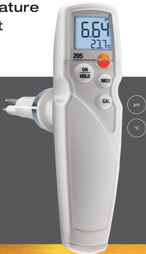
The testo 205 is a robust food penetration measuring instrument for temperature and pH values, with automatic temperature compensation. The robust penetration measurement tip is exchangeable and insensitive to dirt thanks to the hole diaphragm.
